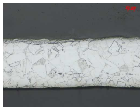
Figure 1. Cross-sectional observations 316L SS 2 mm OD 0.125 mm wall tube sample. Original magnification: 500 x: Detail of the base material
