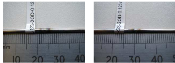
Figure. (a)-(d) 316L SS Tube-Tube weld joints: 2mm OD, 0.125mm Wall
