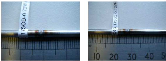
Figure. (a)-(d) 316L SS Tube-Tube weld joints: 3.175mm OD, 0.72mm Wall
