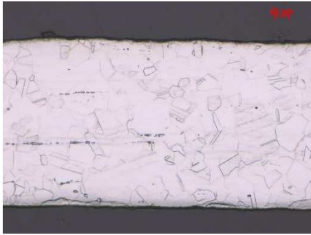
Figure 1. Cross-sectional observations 316L SS 3.175 mm OD 0.22 mm wall tube sample. Original magnification: 500 x: Detail of the base material
